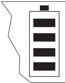
Scales with a built-in battery can work independently from the mains for approximately 30 hours in normal operation. A prerequisite for this is that the background lighting is switched off and that no peripheral devices are connected.
